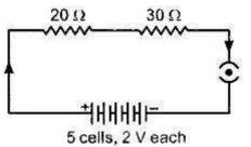
Here, V = 5 x 2 V = 10V, Total Resitance, R =  $20\Omega + 30\Omega = 50\Omega$ Current through both 20  $\Omega$ and 30  $\Omega$ = I =V/R = 10/50 A = 0.2 A Power consumed by 30  $\Omega$  = I<sup>2</sup>R =  $(0.2)^2$  x 30=1.2W
