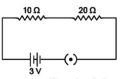
10  $\Omega$  and 20  $\Omega$  are connected in series, their equivalent resistance is
