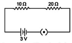
10  $\Omega$  and 20  $\Omega$  are connected in series, their equivalent resistance is
