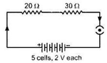
Here,  $V = 5 \times 2 = 10V$ , Total Resitance,  $R = 20\Omega + 30\Omega = 50\Omega$ Current through both 20  $\Omega$ and 30  $\Omega$ = I = V/R = 10/50 A = 0.2 A Power consumed by 30  $\Omega = I^2R = (0.2)^2 \times 30 = 1.2W$
