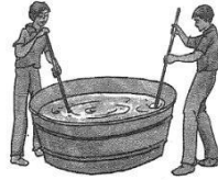
Fig. 3.3. Scouring in tanks
