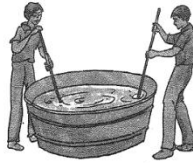
Fig. 3.3. Scouring in tanks
