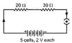
Here, V = 5 x 2 V = 10V, Total Resitance, R =  $20\Omega + 30\Omega = 50\Omega$ Current through both 20  $\Omega$ and 30  $\Omega$  = I =V/R = 10/50 A = 0.2 A Power consumed by 30  $\Omega$  = I<sup>2</sup>R =  $(0.2)^2$  x 30=1.2W
