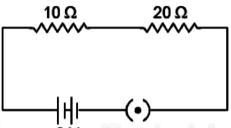
10  $\Omega$  and 20  $\Omega$  are coordered in series, their equivalent resistance is
