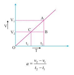
In uniformly accelerated motion, there will be equal increase in velocity in equal interval of time throughout the motion of body.
