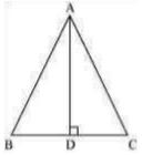
Draw a line segment AD perpendicular to BC. It is an altitude for this triangle. It can be observed that the length of BD and DC is also same. Therefore, AD is also a median of this triangle.
