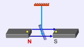
When a paramagnetic rod is freely suspended in a uniform magnetic field, it aligns itself in a direction parallel to the field very quickly.
