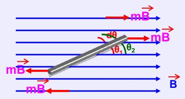
If Potential Energy is arbitrarily taken zero when the dipole is at 90 , then P.E in rotating the dipole and inclining it at an angle  $\theta$  is
