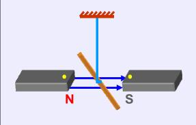
When a paramagnetic rod is freely suspended in a uniform magnetic field, it aligns itself in a direction parallel to the field.
