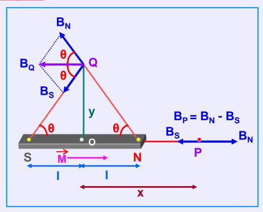
Magnetic Field at a point on the axial line acts along the dipole moment vector.
