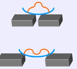
If ferromagnetic liquid taken in a watch glass is placed in uniform magnetic field, it collects at the centre when the magnetic poles are closer and collects away from the centre when the magnetic poles are farther.
