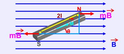
However the forces are along different lines of action and constitute a couple. Hence the magnet will rotate and experience torque.
