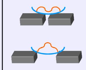
If paramagnetic liquid taken in a watch glass is placed in uniform magnetic field, it collects at the centre when the magnetic poles are closer and collects away from the centre when the magnetic poles are farther.
