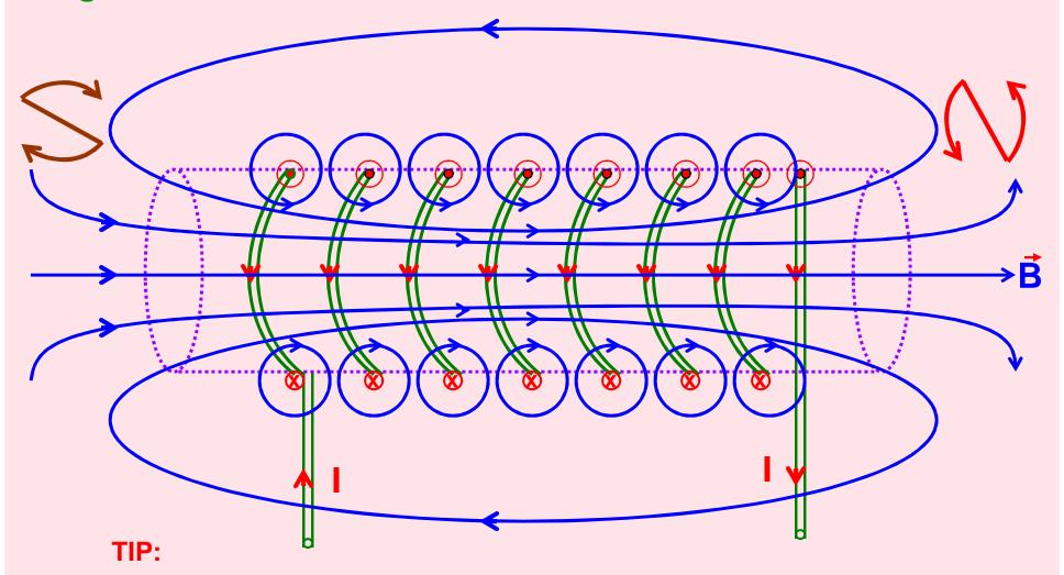
When we look at any end of the coil carrying current, if the current is in anti-clockwise direction then that end of coil behaves like North Pole and if the current is in clockwise direction then that end of the coil behaves like South Pole.
