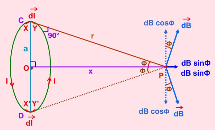
The plane of the coil is considered perpendicular to the plane of the diagram such that the direction of magnetic field can be visualized on the plane of the diagram.
