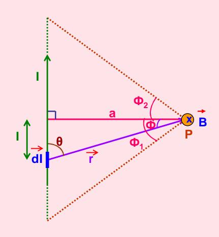
Magnetic field due to whole conductor is obtained by integrating with limits  $-\Phi_1$  to  $\Phi_2$ . ( $\Phi_1$  is taken negative since it is anticlockwise)
