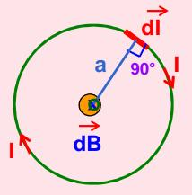
The angle  $\theta$  between dI and a is  $90^{\circ}$  because the radius of the loop is very small and since  $\sin 90^{\circ} = 1$
